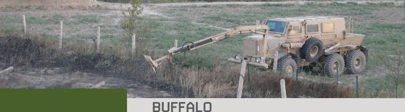
The Buffalo's improvements include increased engine power and greater compatibility, increased driving range, increased fording and slope angle performance, enhanced HVAC and a common spare for all six tires. The enhanced safety features include larger roof hatches for crew egress and both crew and engine compartment Automatic Fire Extinguishing Systems (AFES). With bar armor and air spade as optional features, the more powerful, improved Buffalo is ready to roll.
